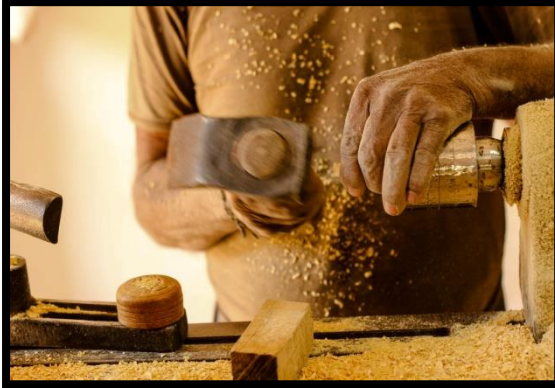
Step 1: Fixing of the wood to the lathe.
